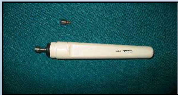
UBM Probe with 50 Mhz transducers.
